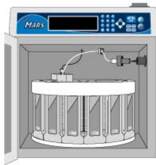
Figure 10. Installed Turntable and Vessels
